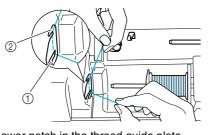
1 Lower notch in the thread guide plate (2) Upper notch in the thread guide plate While holding the thread from the spool in your right hand, hold the end of the thread with your left hand, and then guide the thread through the groove, following the arrows in the illustration.
